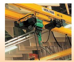
These hoists feature a travelling trolley (for horizontal movement of the load). They are capable of lifting a load of up to 2,000 kg and moving it horizontally in a straight or curved EUROSYSTEM profile.
