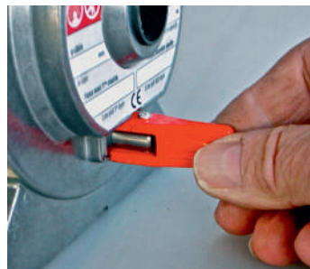
➤ Disengageable drum, no load only.
